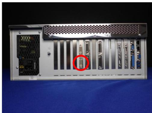
A Matrox P690 card is installed in the Ultima 5M in slot number 10 as counted from the right as shown in the photograph and on Page 2.
