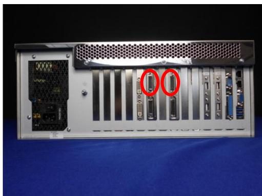
The **upper connectors provide the output ports** as shown in the photograph and circled RED while the lower connectors provide the input ports.
