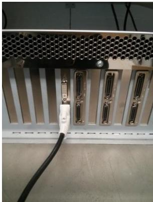
If a Matrox P690 card is fitted, then it will occupy the 5th slot from the left as shown on the left. There are two versions of this card: one with a high density connector requiring an interface cable or one with dual DVI connections (as shown on the left).
