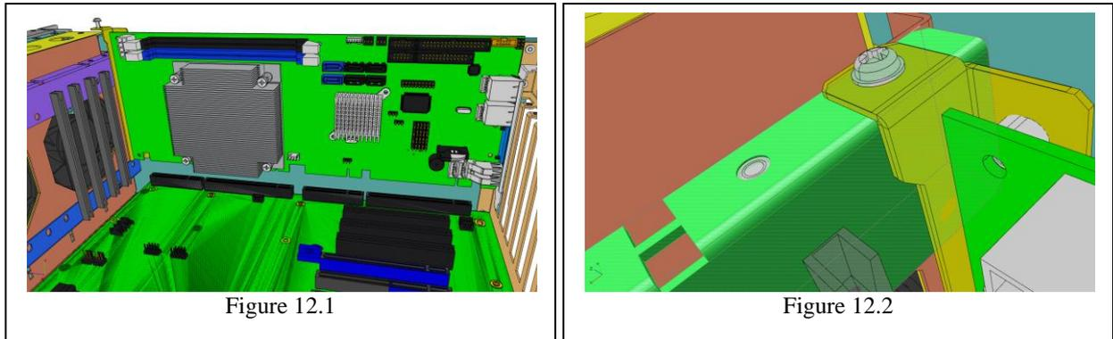
In addition to the retaining screw on the rear panel, the Single Board Computer is held in place with another screw as shown in Figure 12.2.
