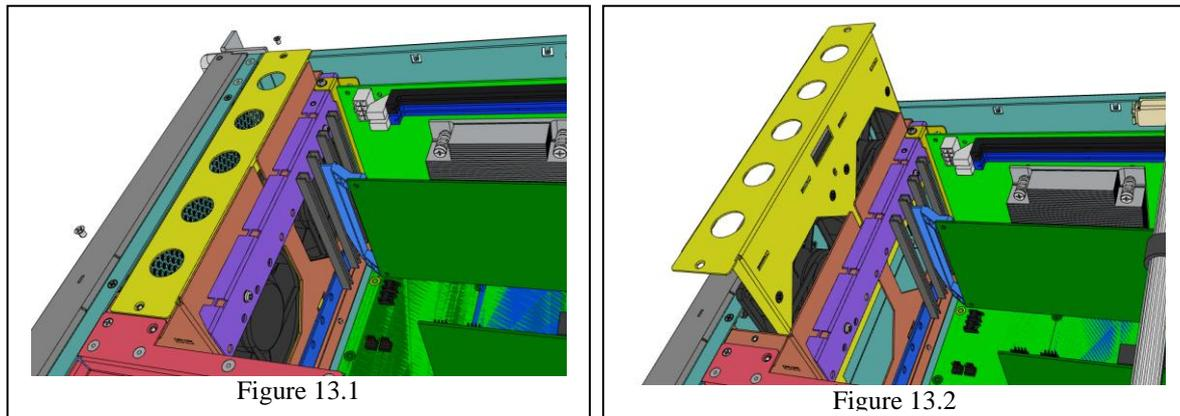
Remove the two retaining screws and pull the fan assembly upwards to remove. Each fan is held in place by 4 screws as show in Fig 13.3 below
