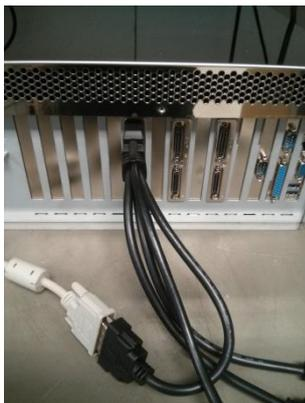
If Matrox Mura cards only are fitted, then the primary display will be output 1 on the left most card fitted. Note that the upper connector is the Output ports, while a lower connector (if fitted) is the Input ports.
