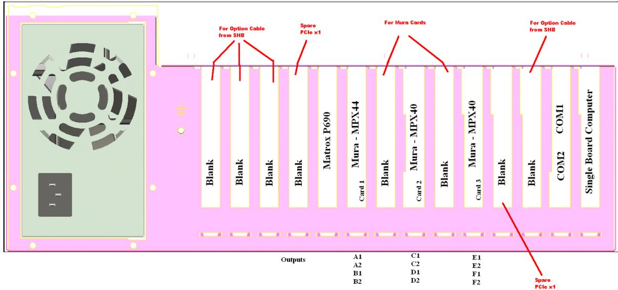
The above picture shows the rear view of the chassis. The Matrox P690 is positioned in PCIe Slot 10 as expected, and the first Mura card is positioned in PCIe Slot 9.
