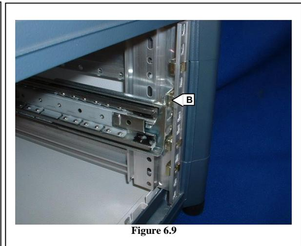
Referring to Figure 6.9, carefully position slide rail and bracket assembly on to fillister screws B at front and rear.
