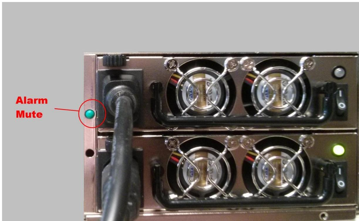
In the event of failure, an audible alarm will sound. This can be cancelled by pressing the Green button shown in the picture above. The faulty module/power inlet will have the LED turned off.
