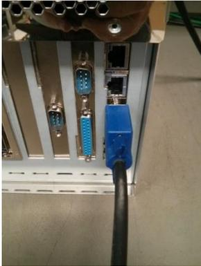
If no additional graphics cards are installed, then the primary display output will be the VGA port on the single board computer, as shown on the left.
