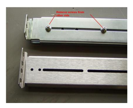
The bolts to be removed are highlighted in the above picture. First turn the bracket over as shown below and extend the slide rail to its full length
