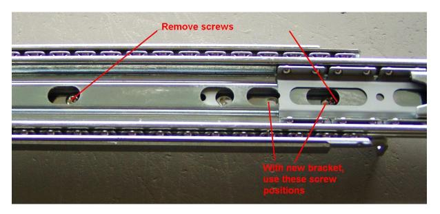
This time the screws are harder to see but with the bracket fully extended they can be accessed. Remove them as before and replace the bracket with the small 4 hole version. Due to the shorter length of the 4 hole bracket, only one screw should be relocated in the same hole with the second screw required to be inserted as shown above.
