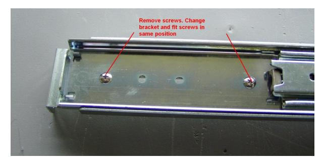
The screws are now visible and can be removed – note the nut on the opposite side may have to be held captive in order to prevent the screw just spinning.
