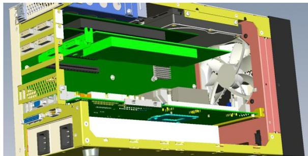
Note that the lower end of the metal bracket has to be pushed into a spring clip just below the level of the back plane. This is designed to improve the EMC performance of the system.
