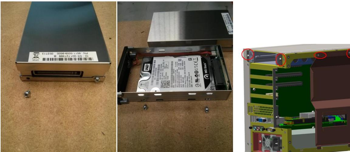
The Caddy base assembly is held in place by 3 screws, two on the rear and one inside. It can then be easily removed or inserted.
