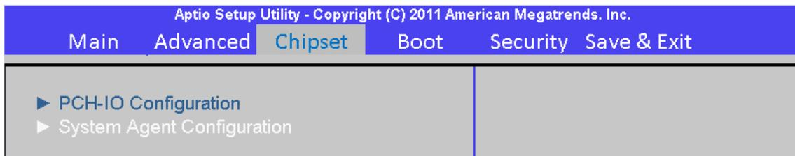
If Matrox P690 and/or Mura cards are installed, it is recommended that the Internal Graphics is disabled.
