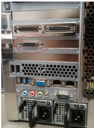
If a Matrox P690 card is fitted, then it will occupy the 3<sup>rd</sup> slot down from the top as shown on the left. There are two versions of this card: one with a high density connector requiring an interface cable (as shown on the left) or one with dual DVI connections.
