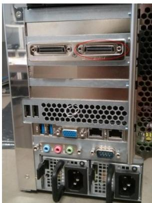
If Matrox Mura cards only are fitted, then the primary display will be output 1 on the lower card fitted.
