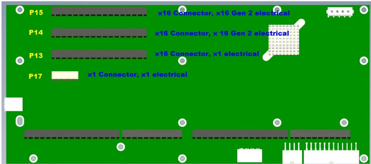
The picture above shows the slot layout on the backplane.
