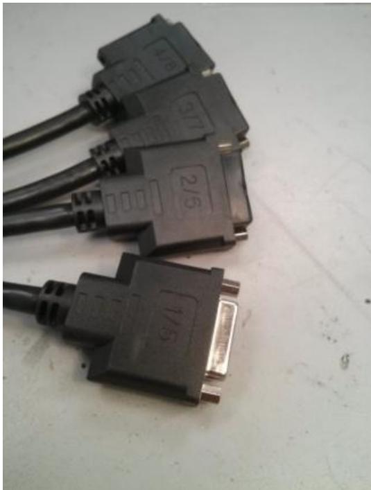
The Four cables are numbered 1/5, 2/6, 3/7 and 4/8. When plugged into the Video Out port of the Mura card, they would be assigned in the Matrox PowerDesk as follows (assuming it is the first Mura card in the system)
