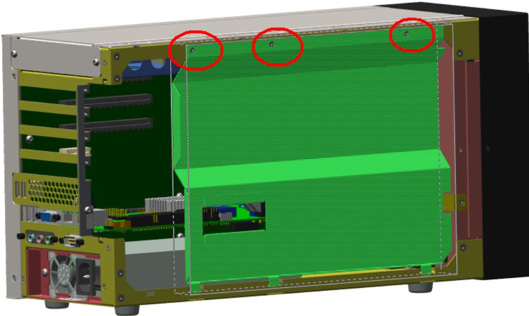
Identify the back plane connector slot to be used. Remove the corresponding blanking plate in the back panel of the chassis by removing the retaining screw and lifting out.
