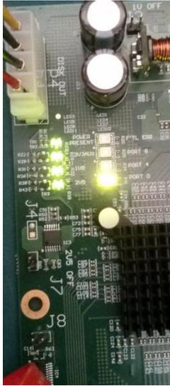
The LED's on the backplane indicate the speed of each PCI Express x 16 slot.
