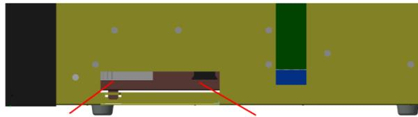
At the rear of the chassis, remove the two screws holding the body of the PSU in place.
