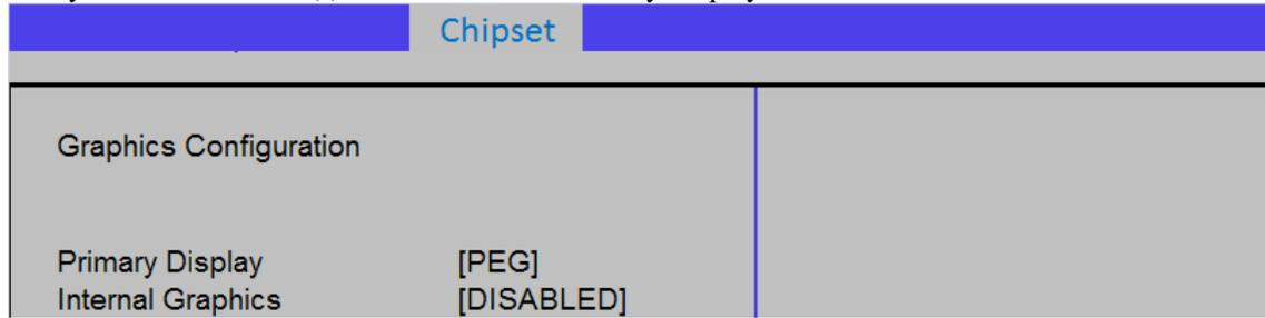
Note that if the wrong display setting is made, it can result in no video being displayed. In this case, to reset to defaults follow the following steps
