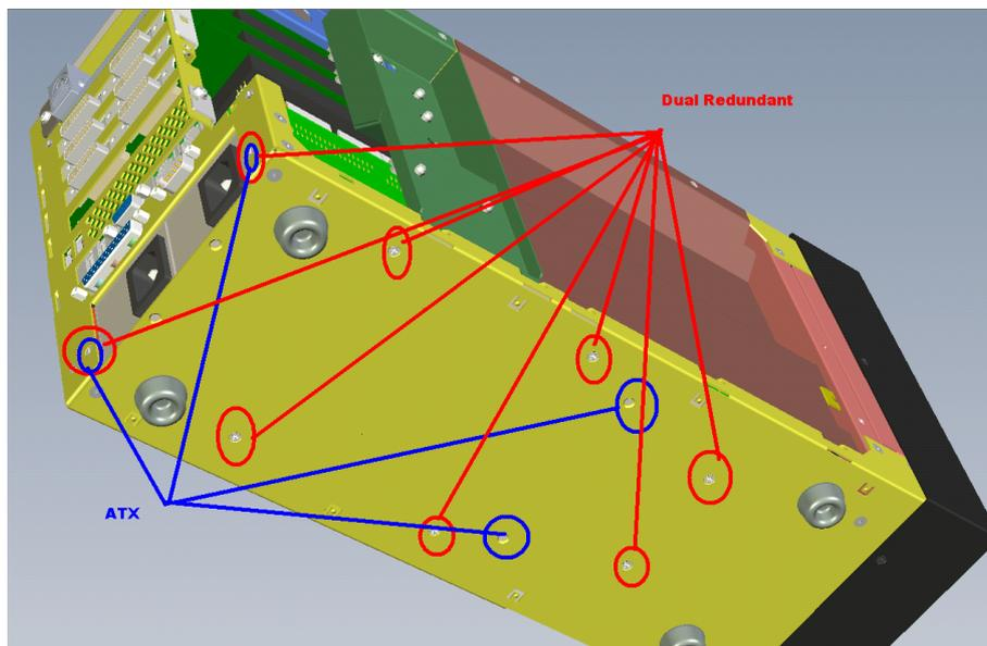
On the underside of the chassis a number of screws will need to be removed depending on the PSU type. For the Dual redundant, there are six screws and for the standard ATX type there are two screws as shown above.
