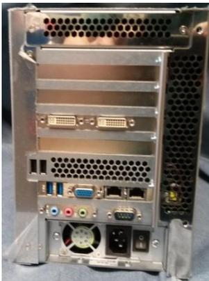
If a Matrox P690 card is fitted, then it will occupy slot number 3 counted from the bottom as shown on the left and on page 2. There are two versions of this card: one with a high density connector requiring an interface cable or one with dual DVI connections (as shown on the left).
