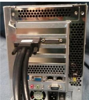
If Matrox Mura cards only are fitted, then the primary display will be output 1 on the card located in slot number 4 as shown. Note that the RIGHT connector is the Output ports, while the LEFT connector (MPX44 and MPX42 only) is the Input ports (shown in picture).
