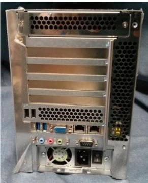
If no additional graphics cards are installed, then the primary display output will be the VGA port on the single board computer, as shown on the left.
