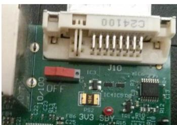
The Slider switch acts as the On/Off button. Slide the switch to the edge of the board to power on.
